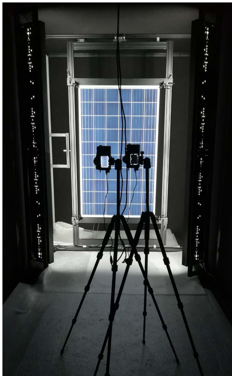
Electroluminescence testing and visual inspection of photovoltaic modules
